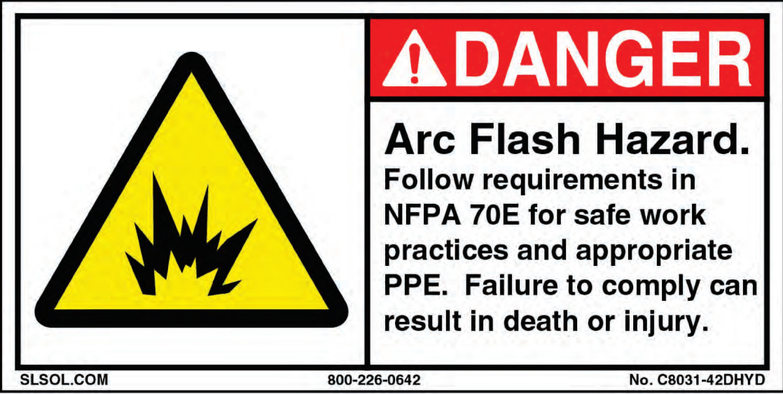
DETAIL ARC FLASH HAZARD WARNING LABEL NOT TO SCALE
